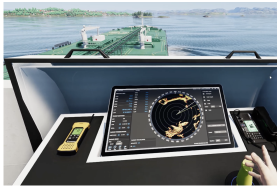
Fig. 6. Standing-out maneuvering panel at the starboard.
